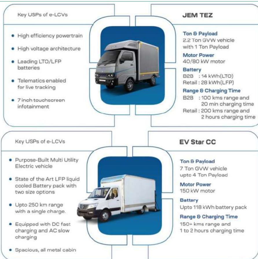
Fig 87: JWL’s electric light commercial vehicle – JEM TEZ
